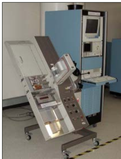
▲ Fig. 6 Gravity-fed auto-handler used in initial high volume switch production.
